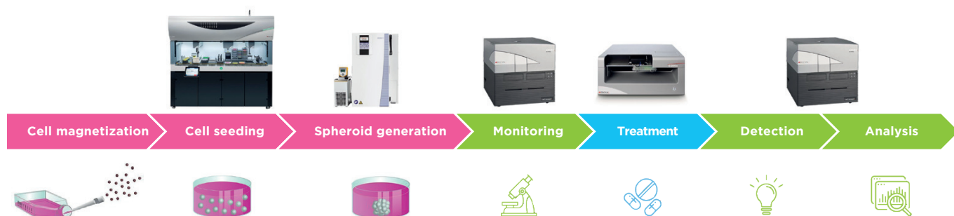
Figure 2: Schematic overview illustrating a drug screening workflow using the Fluent Automation Workstation, D300e Digital Dispenser and Spark Cyto multimode reader.
